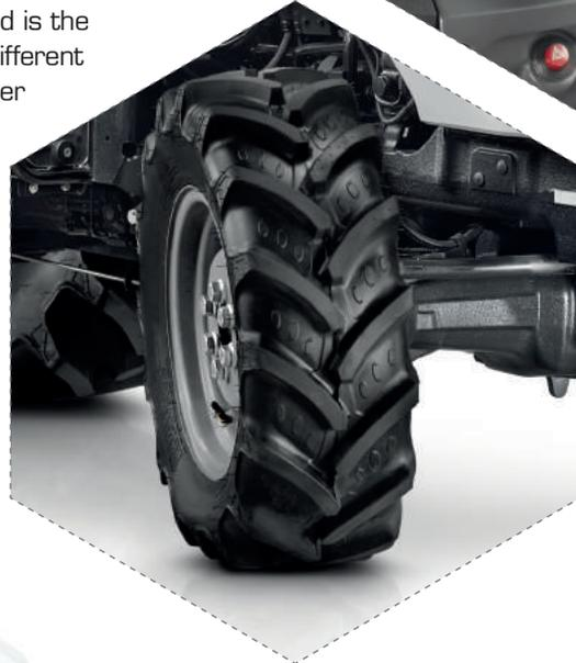
+ **FOUR WHEEL DRIVE AND 100% LOCKABLE DIFFERENTIAL LOCK TO TRANSFER ALL THE POWER OF THE ENGINE EFFECTIVELY TO THE WHEELS.**
