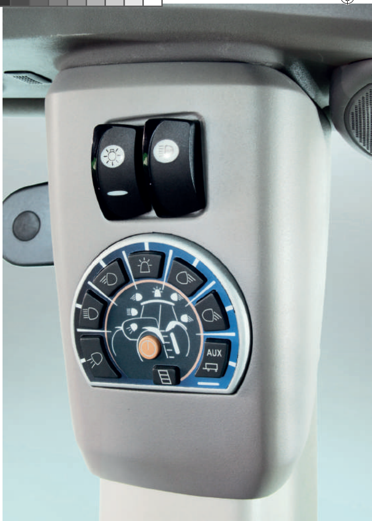
Lights control panel The controls for switching the lights on and off are activated using the Work Operating Light Panel (WOLP), which also lets the driver control the lights mounted on trailers or implements.
