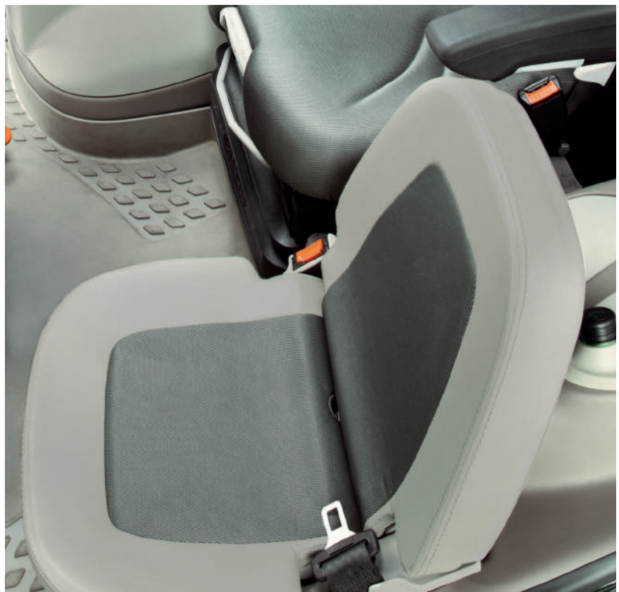
Easy access The comfortable, padded passenger seat folds down to facilitate access to the cab.
